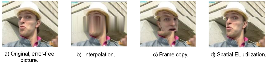
Figure 6. Reconstructed PSNR values: a) 38.2 dB, b) 21.5 dB, c) 23.0 dB and d) 26.6 dB.
